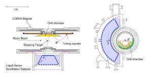
The important part – gradient field COBRA magnet: tracks radius is independent on incident angle at 52.8 MeV/c
